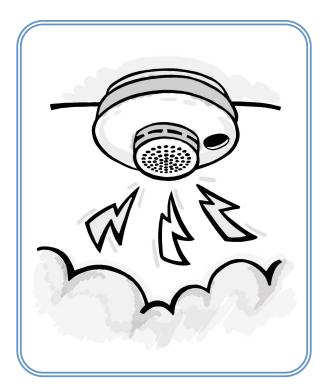
All detecors MUST be on the ceiling-NONE are allowed on the wall!
