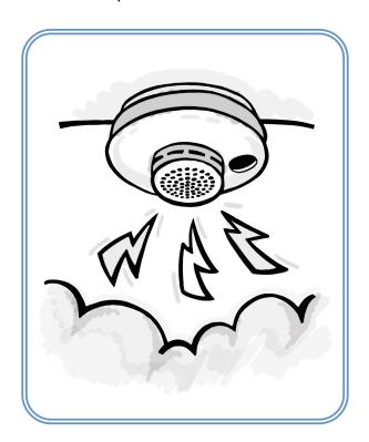
All detectors MUST be on the ceiling—NONE are allowed on the wall!
